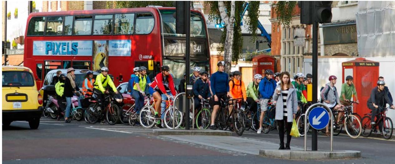
*The available lane widths and position of the central refuge prevents both cyclists and motorcyclists from filtering on the approach to the traffic signals.*
