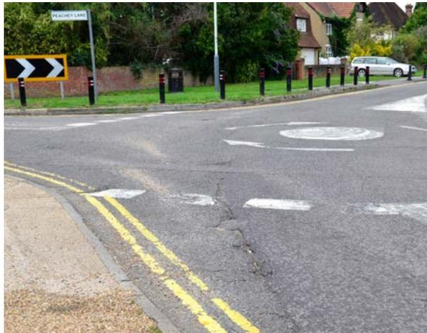
*The owner of the dwelling to the left has treated the run from his private drive to the dropped kerb with gravel (unsealed surface). Vehicle movements from the private drive have transported gravel onto the road, in this case into braking and cornering areas for motorcycles at this mini roundabout.*
