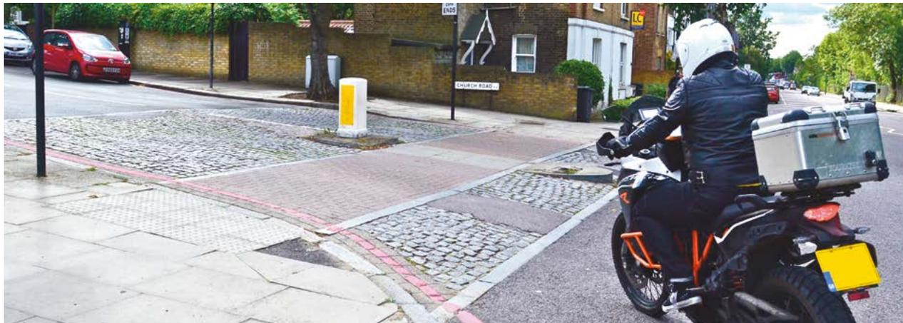
*This entry ramp is set back from the main carriageway, so for a motorcyclist the road surface doesn't change until the manoeuvre is almost completed. However, towards the end of the manoeuvre, on the up ramp, there are potentially slippery granite setts which can cause problems especially when wet.*
