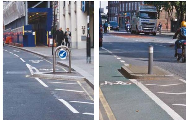
*The build-out forms a strike hazard, with the steel hoop forming an unforgiving structure if hit by a motorcyclist.*
