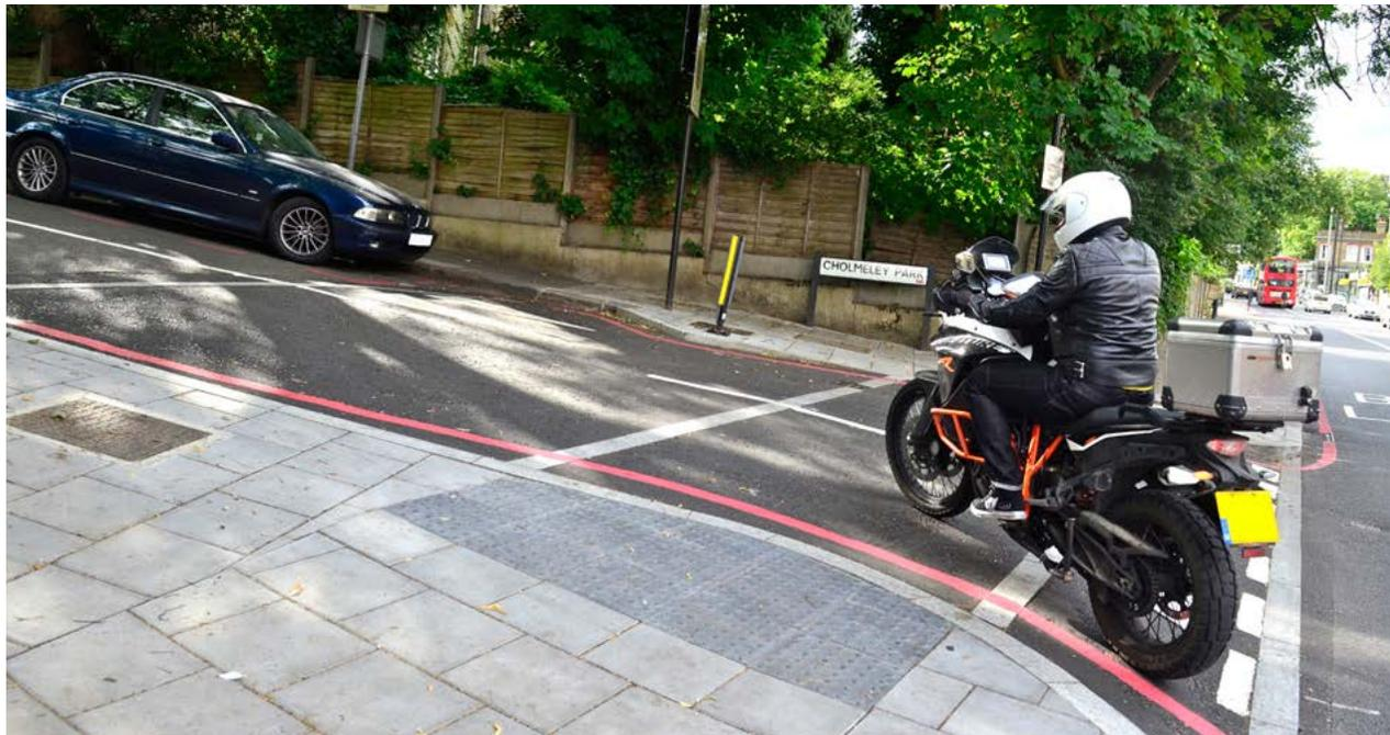
*This example has a good road surface on the up ramp, but the ramp is directly on the border of the main carriageway and has a gradient of 1 in 5, which can cause problems for motorcyclists.*
